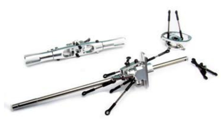
One of the heads, the mast assembly and a swashplate, as they come out of the box
