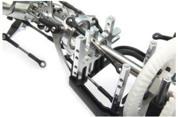
The upper bearing block and the servo rails
