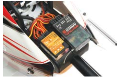
A Microbeast unit was mounted alongside the Spektrum receiver
