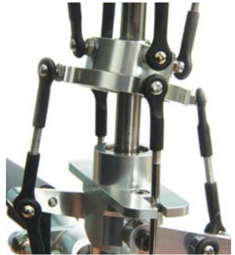
Look closely and you can see the upper plastic ball link starting to bend – it's unlikely to get that far in flight
