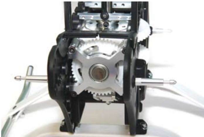
The reduction gearbox installed, ready for the motor to slide in behind
