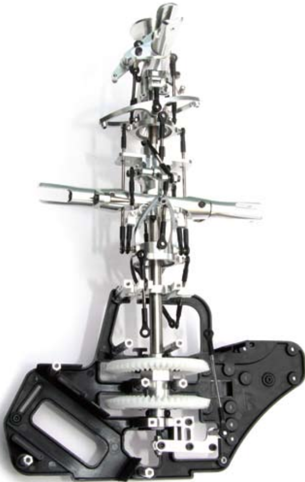
The heads, masts and main gears laid into the right side frame – it's a perfect fit
