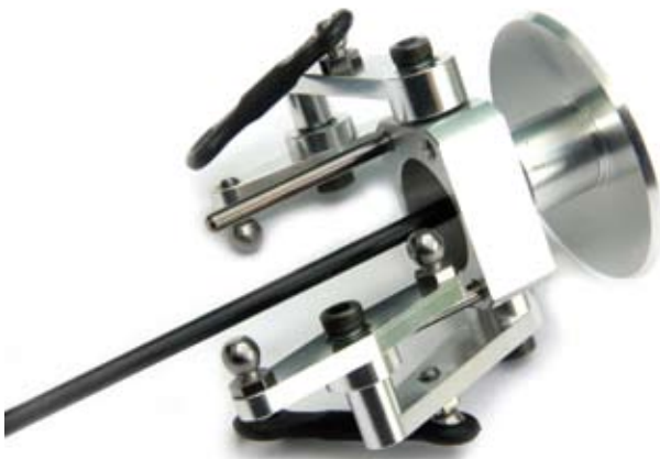
The yaw washout unit fits over the top head and adjusts the top head collective pitch for yaw control...
