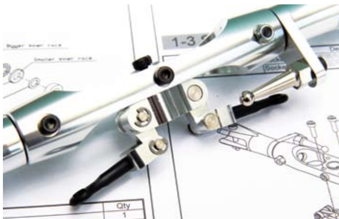
Each head has a swashplate driver bolted on, note the two cross bolts which act as flapping pivots
