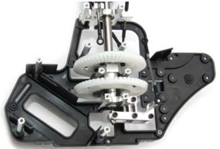
A view of the yaw control lever under the main gears
